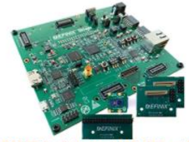
Featuring T120 FPGA with hardened MIPI CSI-2 and DDR DRAM
