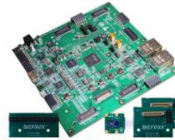
Featuring T120 FPGA with hardened MIPI CSI-2 and DDR DRAM
